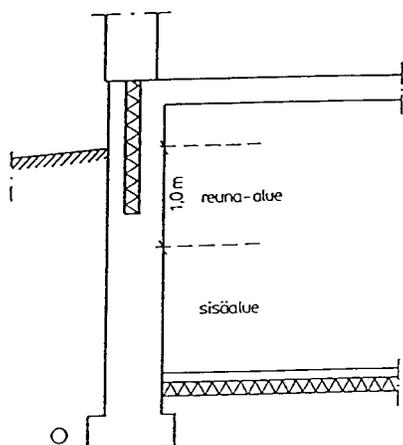
Figure 3. Division of the part of a wall against the ground into zones
