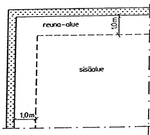
Figure 1. Division of the base floor against the ground into zones
